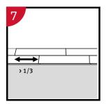
Staggered joint distance i.e. minimum distance between short ends of planks in parallel rows shall not be less than 20 inches.
