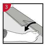
When folding the plank down it is important to start from the corner closest to the previous row, folding down towards the centre, and continuing towards the opposite long side. During the fold down, make sure the planks are close to each other.
