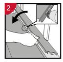
Remove the vertical locking part of the strip with a chisel, put applicable glue on the strip and push the planks horizontally together. Place some spacers between last plank and the wall.
