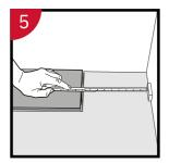
At the end of the first row, put a spacer against the wall and measure the length from the last plank to the wall.
